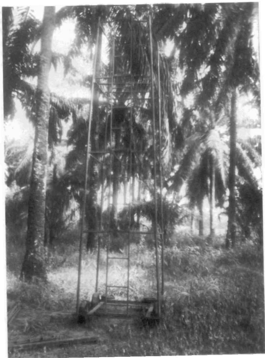
Plate 23: The support mechanism for usage of motorised palm bunch harvester
