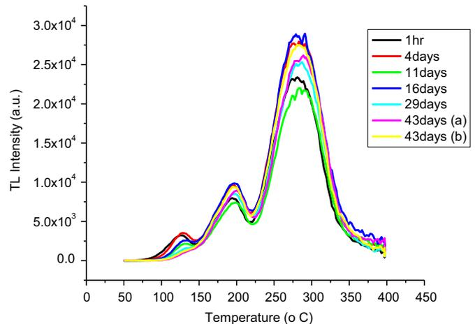
Fig. 3. Glow curves of fluorite irradiated to the dose of 43.2 mGy and read at the heating rate of 5 °C s<sup>-1</sup> for different storage periods at room temperature.
