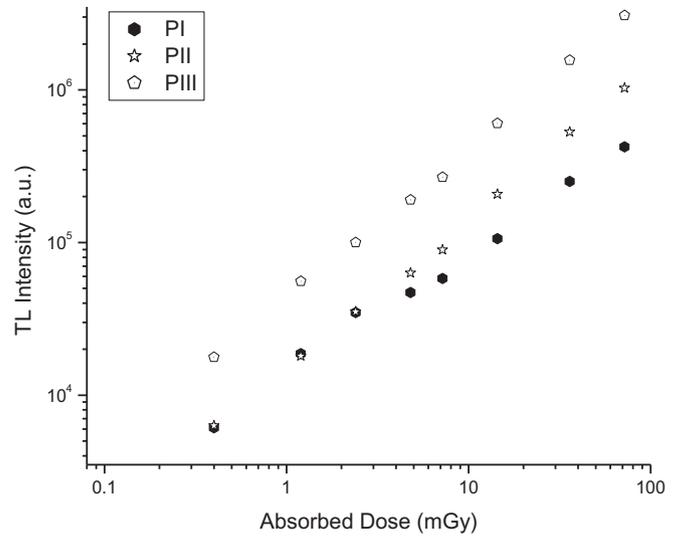
Fig. 2. Dose response curves of the observed peaks (PI, PII and PIII) of fluorite in the absorbed dose range of 40 μGy–72 mGy.
