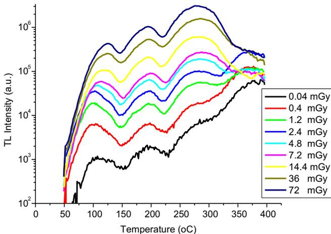
Fig. 1. Glow curves of fluorite in the absorbed dose range of 40 μGy–72 mGy acquired at the heating rate of 5 °C s<sup>-1</sup>.
